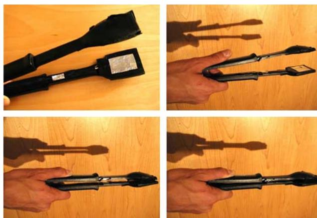
**Figure 7: Doubly sensed tongs:** (top right) Two foil sensors detect weak and strong grabs with the tongs. The tongs have three states: open (top right), weakly closed (bottom left) and strongly closed (bottom right). Weakly grabbing a base moves the whole molecule, strongly grabbing a base moves only it. Grabbing empty space with the tongs moves the whole scene, grabbing empty space twice (there are two sets of tongs) activates combine scaling, translation, and rotation.
