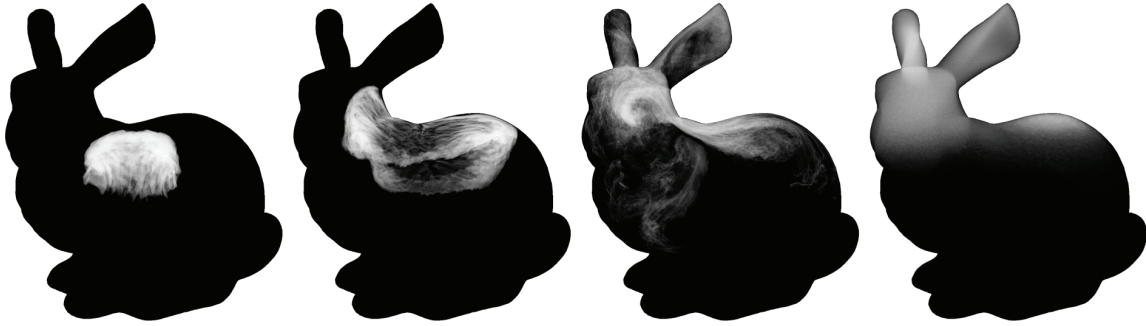
Figure 1: Discrete Fluids : we present a novel geometric integration scheme for fluids applicable to tetrahedral meshes of arbitrary domains. Aside from resolving the boundaries precisely, our approach also provides an accurate treatment of vorticity through a discrete preservation of Kelvin’s circulation theorem. Here, a hot smoke cloud rises inside a bunny shaped domain of 7K vertices (32K tets—the equivalent complexity of a regular 19^3 grid), significantly reducing the computational cost of the simulation for such an intricate boundary compared to regular grid-based techniques (0.47s/frame on a Pentium 4, 3GHz).
